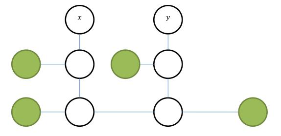
We have 2 new nodes per each variable-node (x, y, ...), and in addition we have the green node from before, here represented as different nodes (but they are all the same one).
