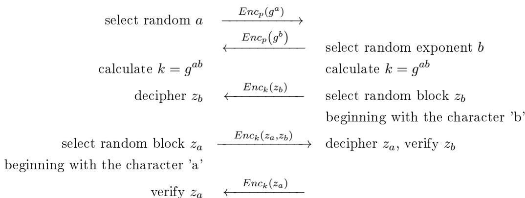
If verification fails, the protocol is immediately aborted. Pru can also halt all communication for a few minutes, fooling Alice and Bob to think that the other side has had a power outage, so Alice attempts to re-establish a connection to Bob and to renegotiate keys. Unless errors (connection or verification) happen a lot, Alice and Bob do not suspect.
